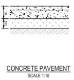
150MM SLAB, REINFORCED WITH 5L42 MESH POURED ON 100MM SAND BLINDING OVER WALKER PROOF MEMBRANE ON 100MM ASPHALT COMPACTED TO 98% CBR. INCREASE SLAB THICKNESS TO 200MM FOR AT LEAST 15M FROM THE ENDS.
