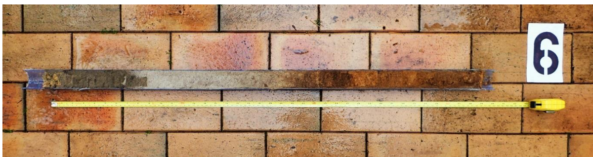
Figure 12. Core 6, Cronulla High School, Cronulla, central eastern New South Wales (56H 329982.759 6231979.364). Surface elevation 5.237 m AHD. Note that the 0.05 m of concrete that forms the upper unit at the site was removed before coring.
