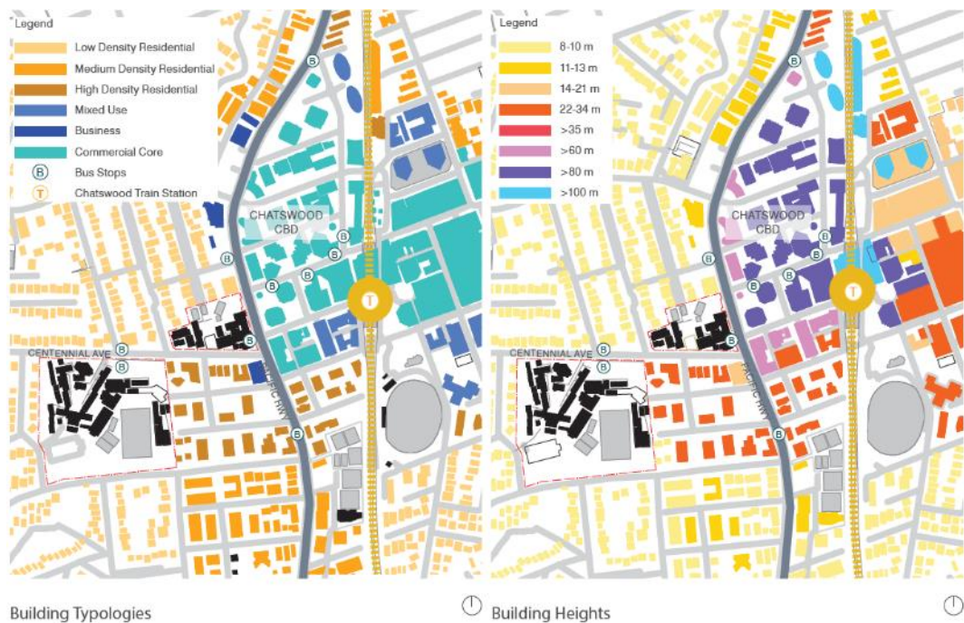
Figure 9 Building Typologies and Heights (Architectus)
