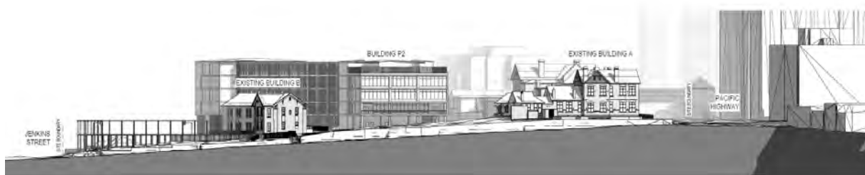
Figure 82. Centennial Avenue street elevation, showing the existing Buildings A and B on either side of the school boundaries. The proposed Buildings P1 and P2 are visible in the centre and behind Building B. The undercover carpark and sports court are visible to the left of Building B. Source: Architectus, 'Street Elevations,' Drawing No. SD-BX-A2000, Issue B, 25 th November 2019.
