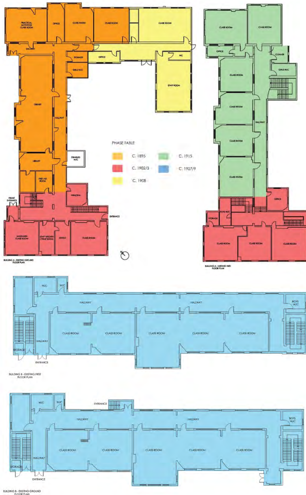
Figure 13 Floor plans of Buildings A (top) and Building B (bottom) illustrate the phases of construction of the two buildings considered to be of heritage significance. Source: Nimbus Architecture and Heritage.
