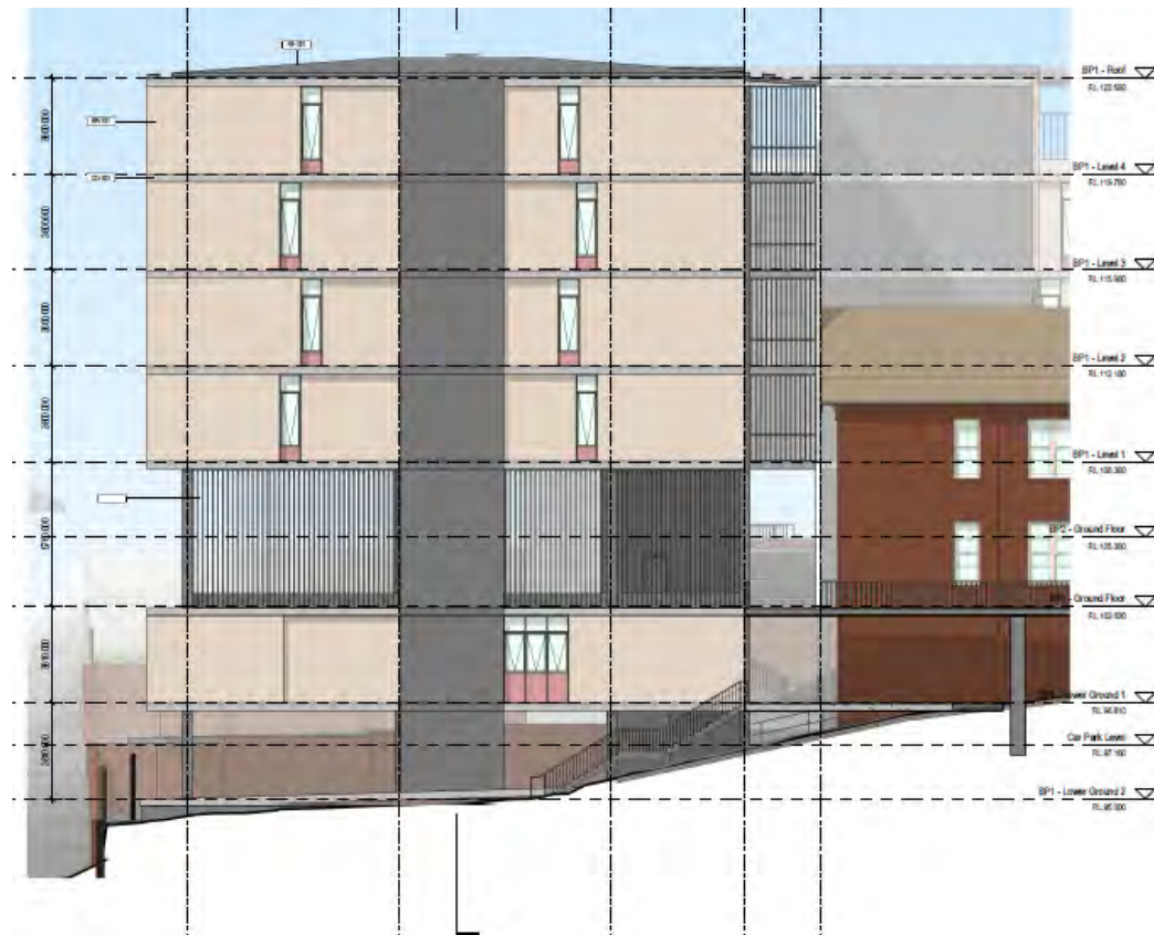
Figure 86. Elevations - Sheet 4 – P1, showing the western elevation of proposed building P1 looking towards east. Proposed building P2 is also visible behind building P1 as well as heritage building B to the front. Source: Architectus, 'Elevations – Sheet 4 – P1,' Drawing No. SD-BP-A2003, Issue A, 29 th November 2019.
