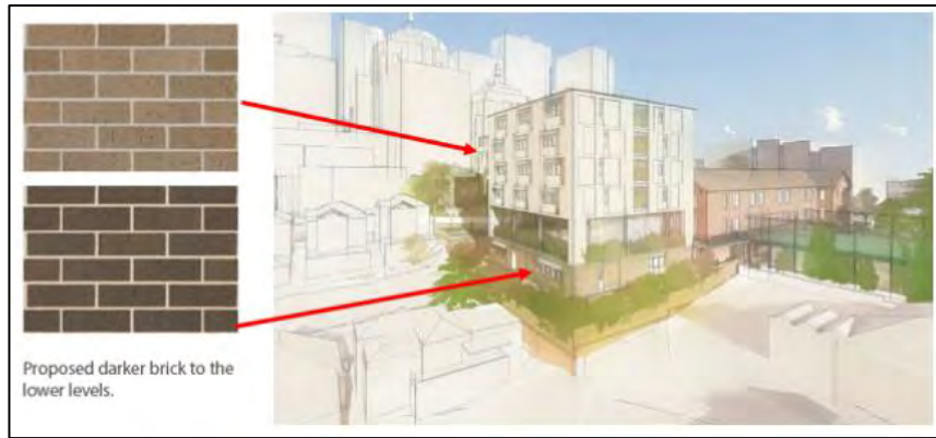
Figure 41 | Proposed darker and lighter coloured bricks for Building P1 facade (Base source: RtS 2020)
