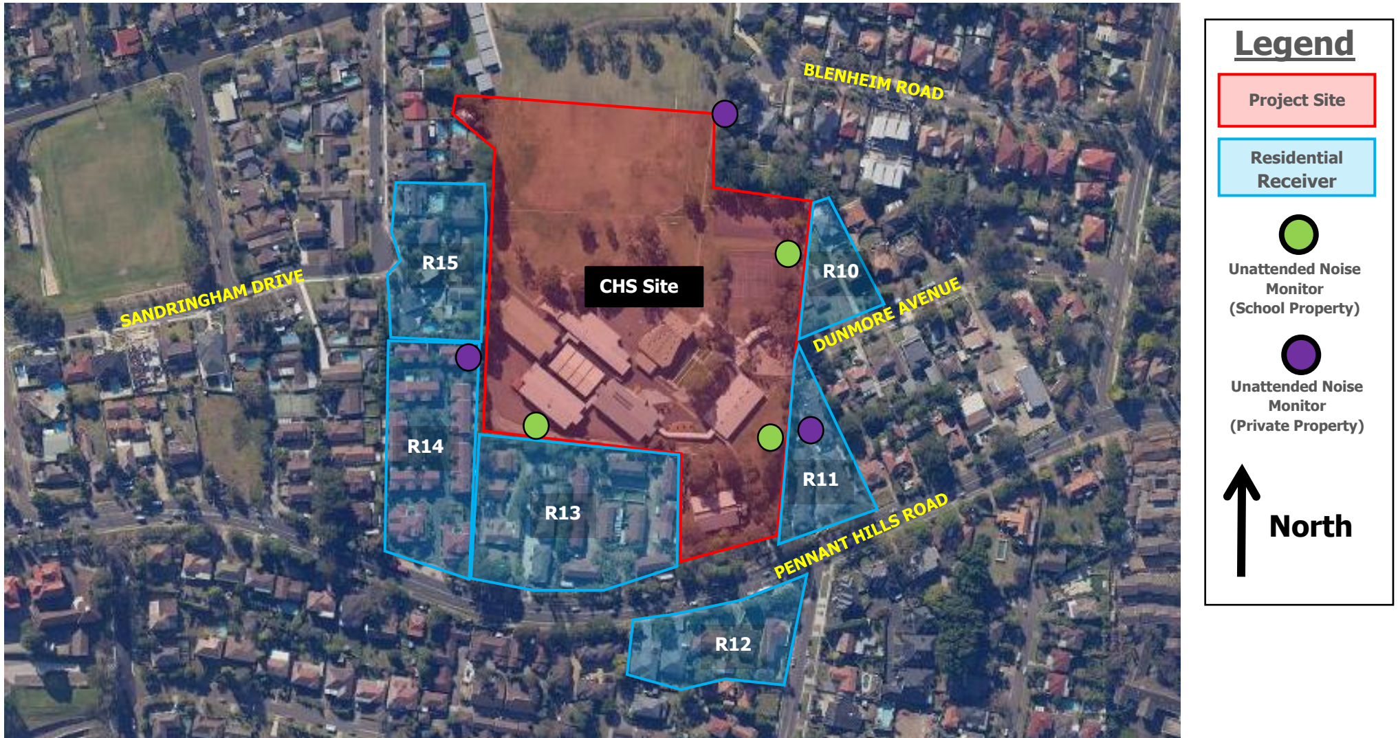
Figure 3 Site Map, Measurement Locations and Surrounding Receivers Cumberland High School (CHS) – Sourced from SixMaps
