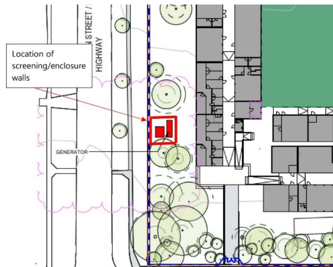
Figure 1: indicative location of the temporary generator.
