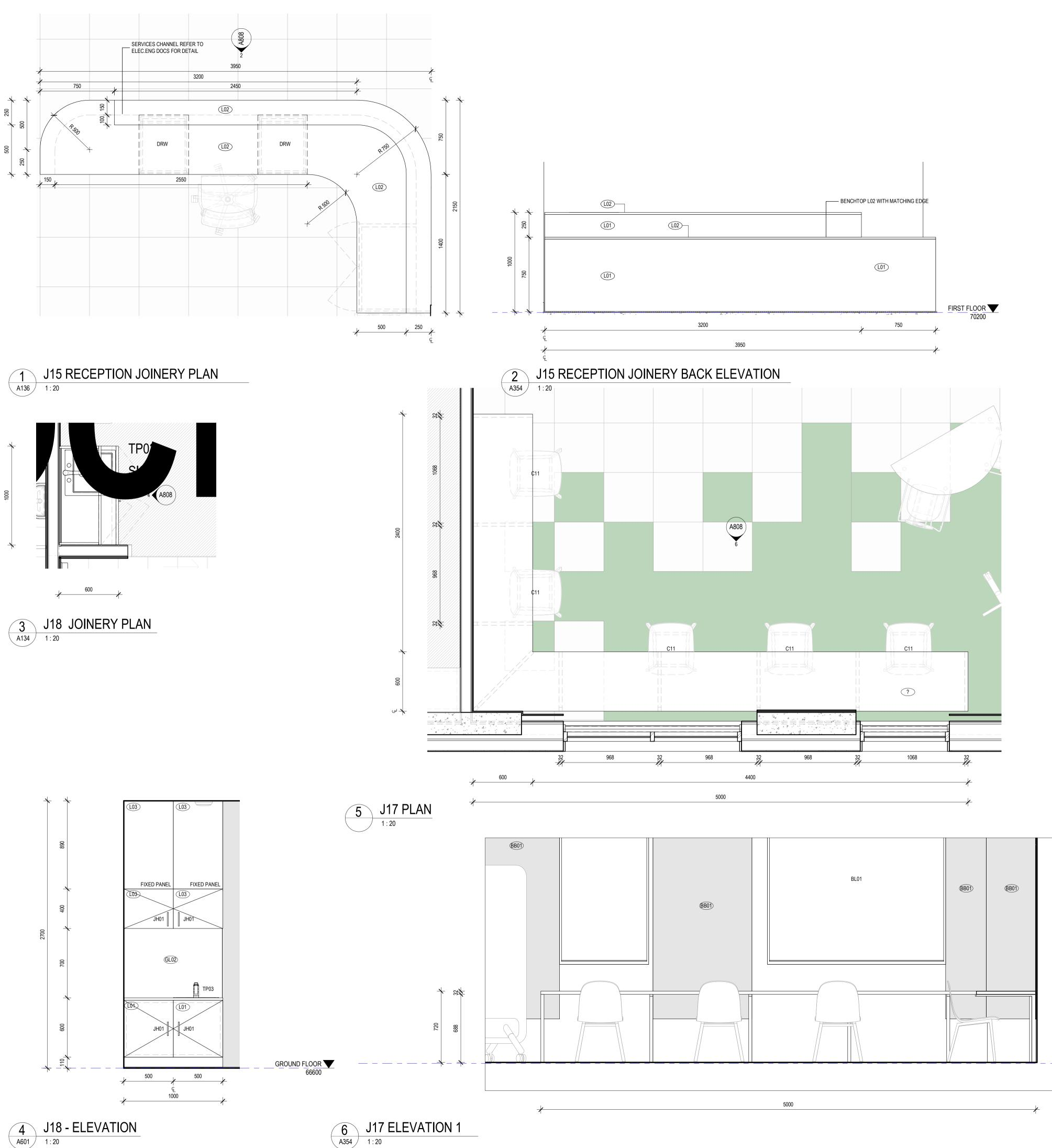
JOINERY UPSTAND AROUND PERIMETER OF BENCH TO WALL. ELECTRICAL OUTLETS TO BE FLUSH FIXED TO UPSTAND.
