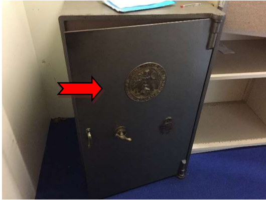
Photograph 7: Asbestos containing fibre cement.
