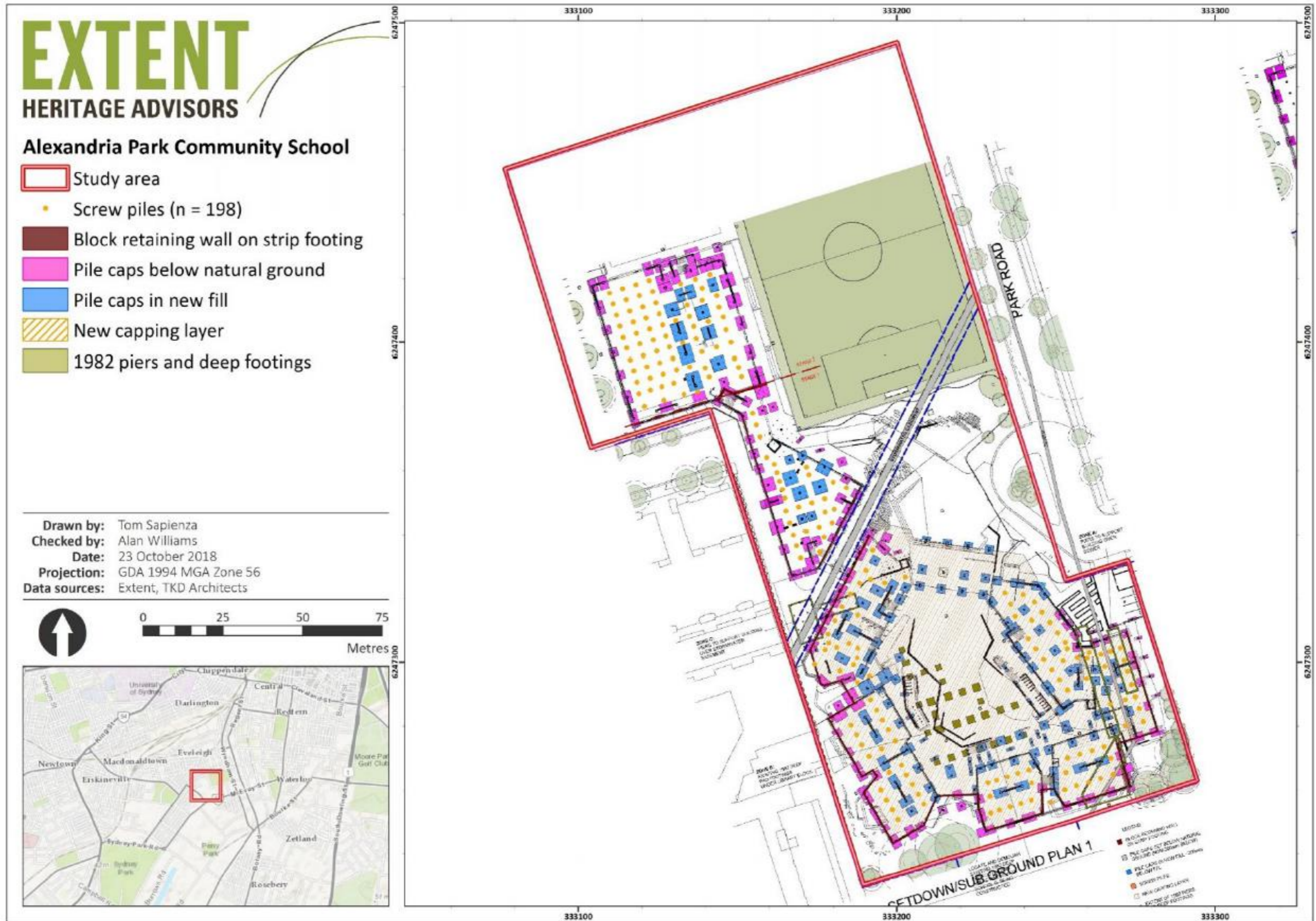
Figure 3.2 The proposed screw piling locations, capping layer and pile caps for the Alexandria Park Community School. Extent Heritage Pty Ltd (2018), Figure 3 in original report.
