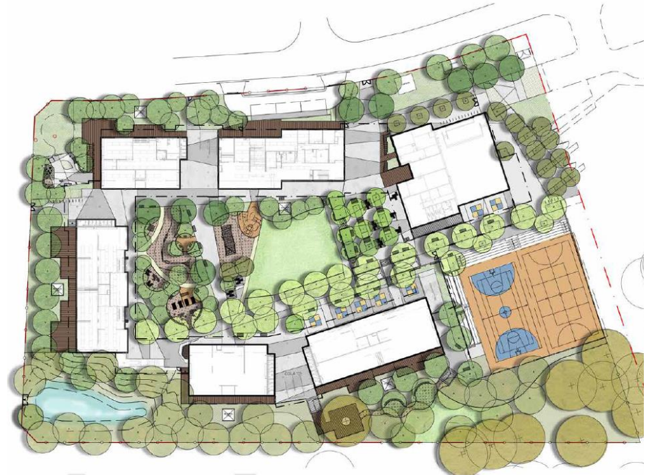
The site plan for the proposed new school building at 10000 Farmland Drive shows a complex layout with five main building blocks and various outdoor spaces. The buildings are labeled as follows: BLOCK B1 LEARNING SPACE PTL 45.50 BLOCK A LIBRARY / GYM PTL 45.50 BLOCK C COMMONS HALL PTL 45.50 BLOCK B2 LEARNING SPACE PTL 45.50 BLOCK B3 LEARNING SPACE PTL 45.50 BLOCK D LEARNING SPACE PTL 45.50 COMMONS HALL PTL 45.50 The plan also includes a large central green area, a basketball court, and a playground. Landscaping includes numerous trees and shrubs. The site is bordered by Farmland Drive to the north and a parking lot to the west. A north arrow is located in the bottom right corner.
