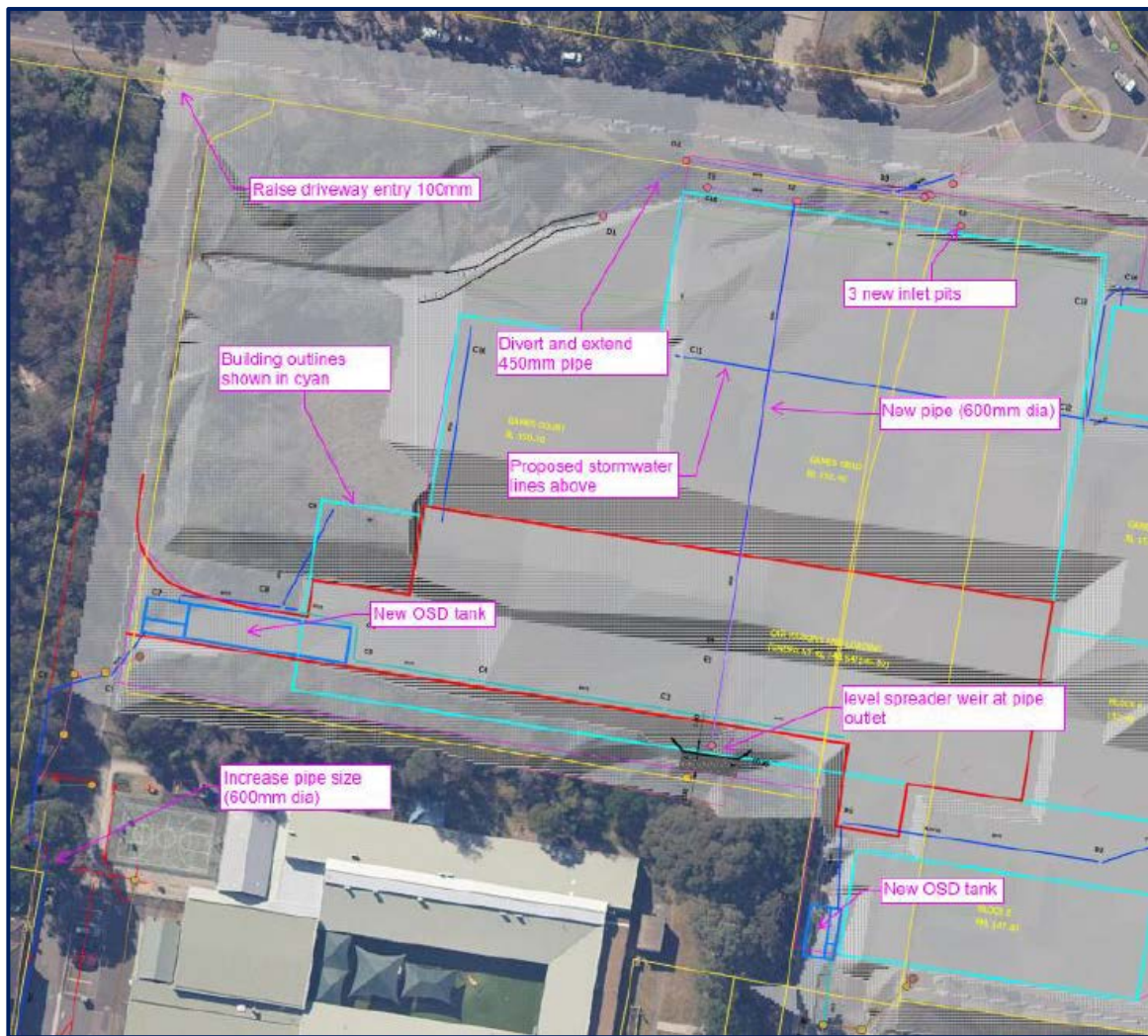
Figure 29 | Proposed flood mitigation works (Source: updated Civil Engineering Report, October 2023)
