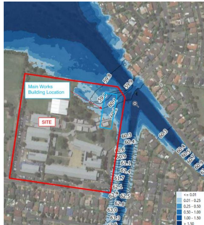
Figure 6: PMF Flood Extent and Levels (Source: Enstruct)
